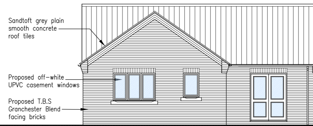
Proposed Rear Elevation 1:100
